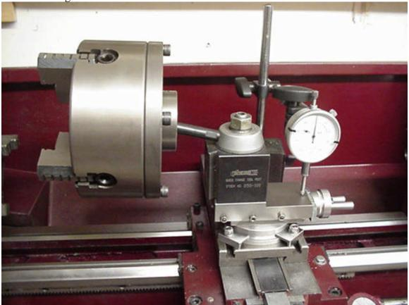
The new mounting system attributes its stiffness due to the major components being in compression and a much wider supporting area.
